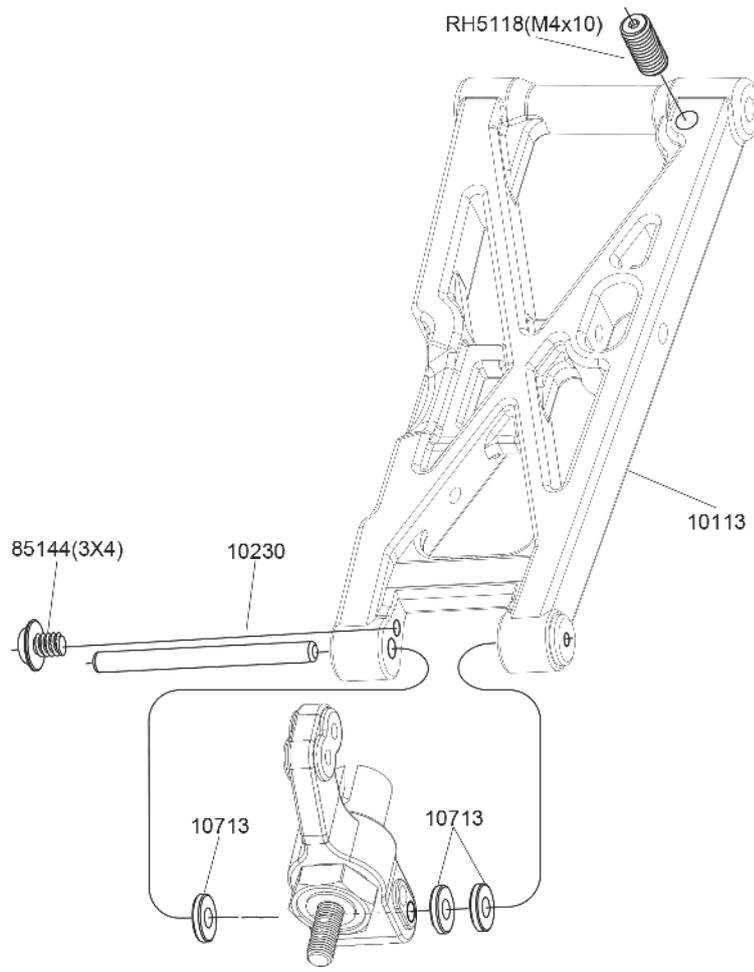
Assembly rear hub carrier set with rear lower susp arm.
