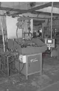
CNC For Pin Hole Drilling Of Cylinder Plug And Casing
