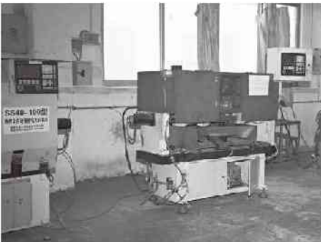
CNC For Plug Hole Drilling Of Cylinder Casing
