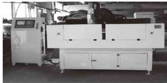
CNC For Hole Drilling Of Trim
