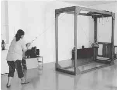
Horizontal Impact Test
