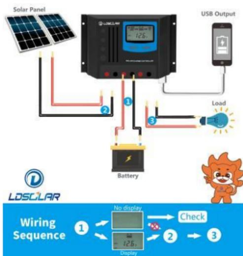
Connect the system in the order of **①** battery (after connected the battery, the LCD will be on. If LCD not on, stop connecting, and check whether the positive and negative poles are reversely connected. Only after the LCD displays, you can continue to the next step. Always connect the battery first, in order to allow the controller to recognize the system voltage) **②** PV array **③** load and disconnect the system in the reverse order **③②①**.
