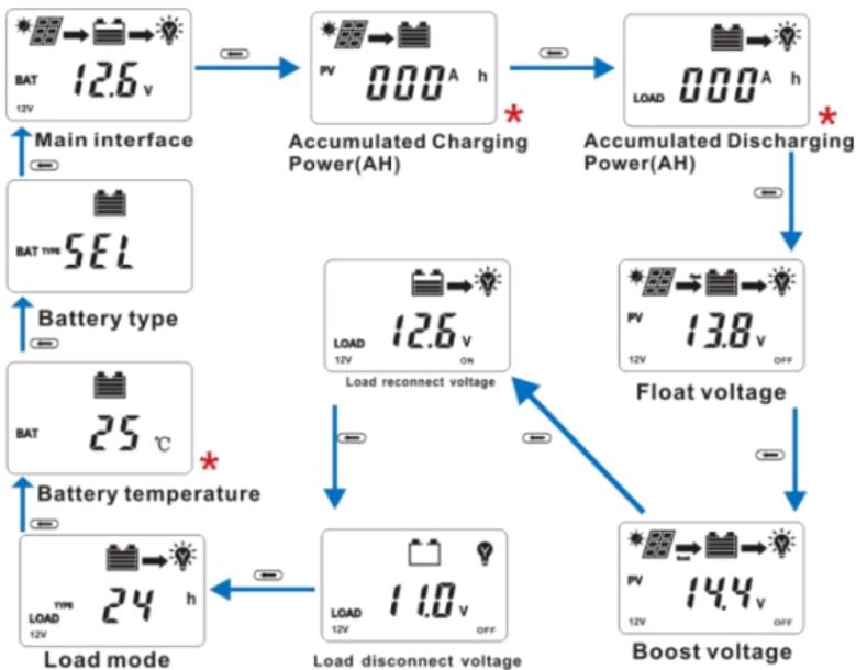
The interfaces marked “\*” are not equipped for SD2410C,SD2420C and SD2430C.
