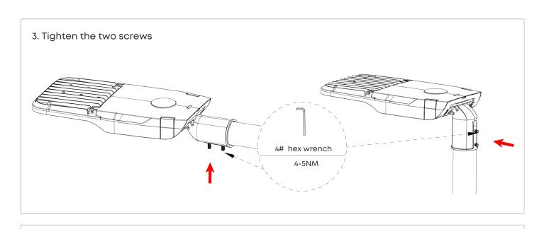
4. If angle adjustment is required, loosen the two screws by 2-3 turns, ensuring they are not completely removed. Proceed to align the component before retightening.
