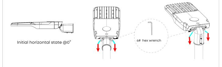
5. Rotate the fixture to the proper angle based on the actual requirement, then tighten two screws behind the fixture on the bracket.
