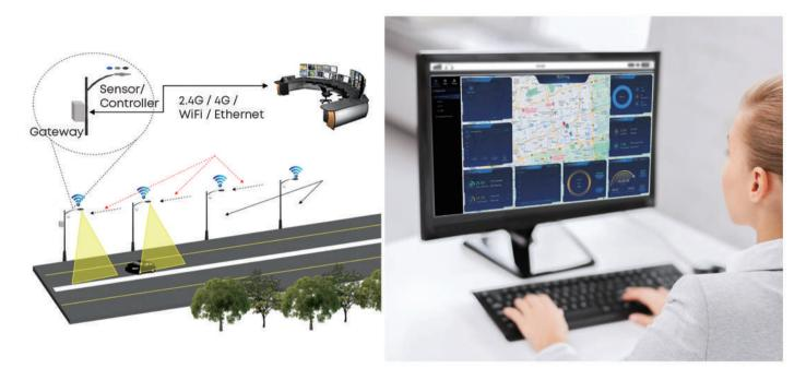
By using the cloud platform, the control center manages group switching period, dimming, data, status, monitoring, etc
