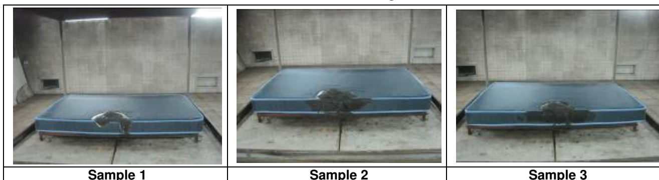
PHOTO 2. Mattress After Testing To 16 CFR 1633
