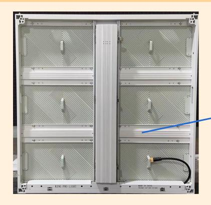
The full-profile aluminum cabinet improves the cabinet's corrosion resistance, reduces the cabinet's weight, reduces the cabinet's thickness, and improves the cabinet's accuracy.
