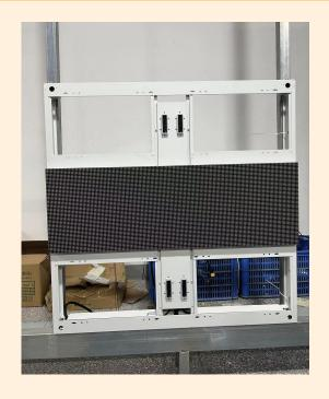
Step 1 :First remove the modules in the first and third rows of the cabinet.
