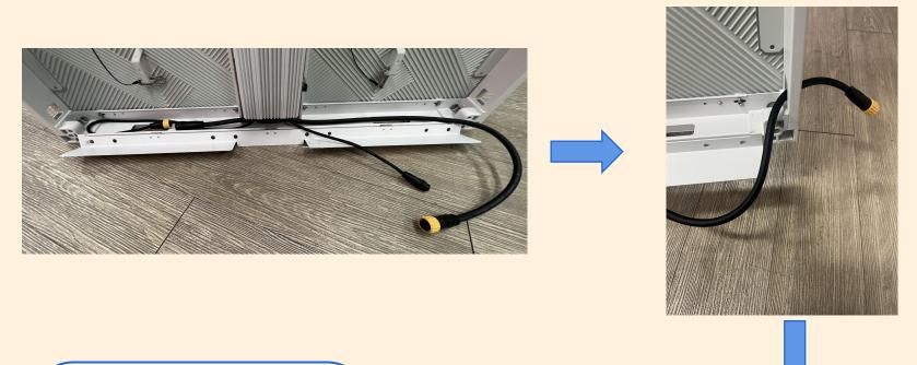
Step 2:Open the power cord and network cable protection slot, pass the power cord and network cable through the cabinet wiring holes, and then connect them.
