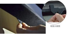
2.Gently lift the bottom of the screen, use the bottom mounting bracket to hook the groove of the screen.
