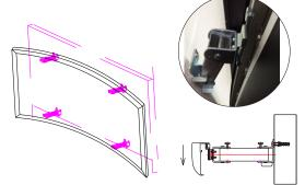
3. Mount the screen onto the brackets.
