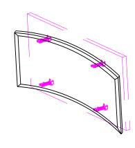
5. Push the frame to rotate the mounting brackets, adjust the screen to the suitable position.
