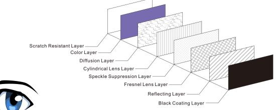
Black Technology III: high gain, speckle suppression INP-FNE has 1.2 Gain, 50% higher than similar projector screens. It can effectively eliminate speckles and protect human eye.
