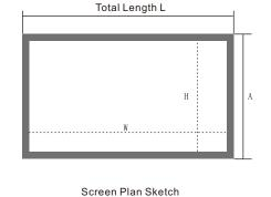
Viewing Area Format Size Total Length L(mm) | Total Height A(mm) W (mm) \*H (mm) 871 70" 1549 1771 996 1891 1116 16:9 100" 2213 1245 2333 1365 120" 2656 1494 2776 1614 1625 1219 1745 1339 4:3 100" 2030 1520 2150 1640 2440 1830 2560 1950 120" Other sizes can be customized
