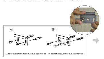
1.According to the quantity of the mounting brackets and appropriate distance, you should install the mounting brackets at suitable place on the wall with screws .
