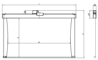
Large Roll Down Motorized Screen UC3(Wirerope Type)
