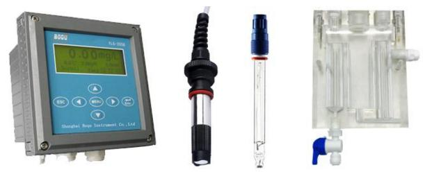
YLG-2058 Industrial Online Residual Chlorine Analyzer is two channels to measure pH and chlorine; It is a high-intelligence on-line monitor, It is made up of three parts: a secondary instrument and a sensor, a organic glass flow cell. It can measure residual chlorine, pH and temperature simultaneously. widely used for continuous monitoring of residual chlorine and pH value of various water quality in power, water plants, hospitals and other industries.
