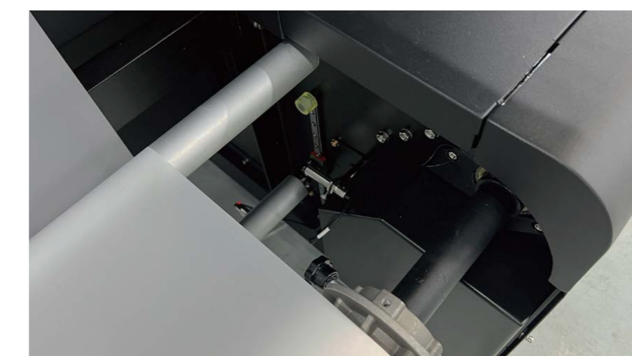
Upgraded tension rod system supporting 100–300m film rolls
