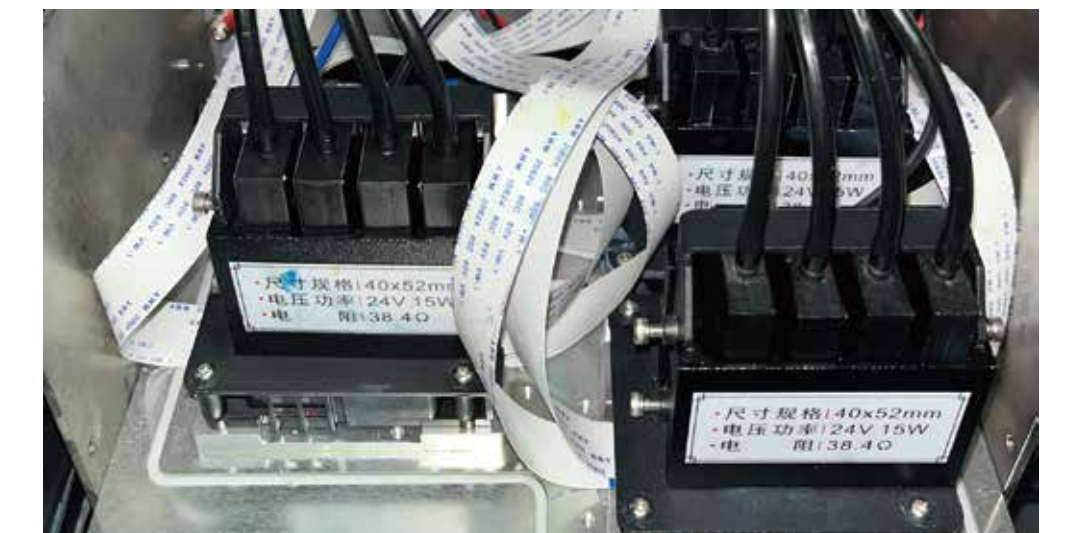
Base plate and damper heating
