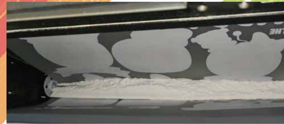
Powder stopping rod to make sure even powder supply
