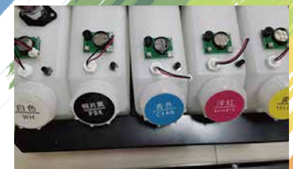
Inktank arlam device Monitor the ink lacking in tank
