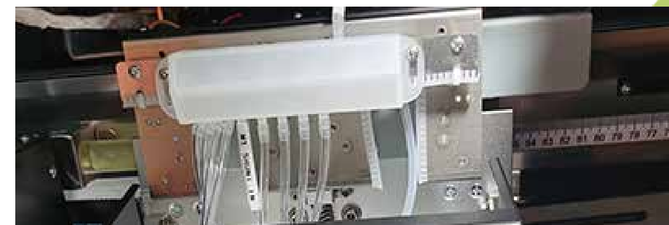
Ink shunt :avoid of ink bubbles to print smoothly
