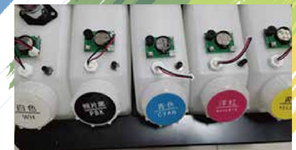
Inktank arlam device Monitor the ink lacking in tank.
