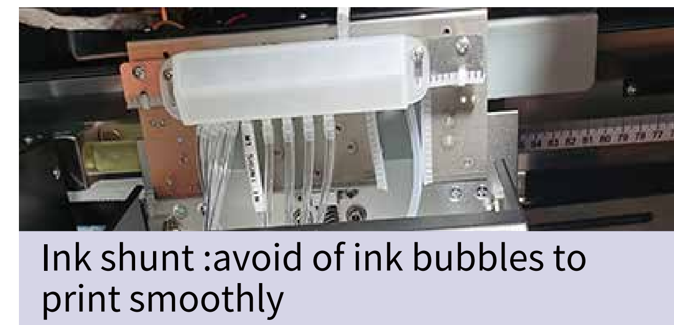
White ink stirring and circulation system Stirrer : avoid of head blocking Ink tank alarm device
