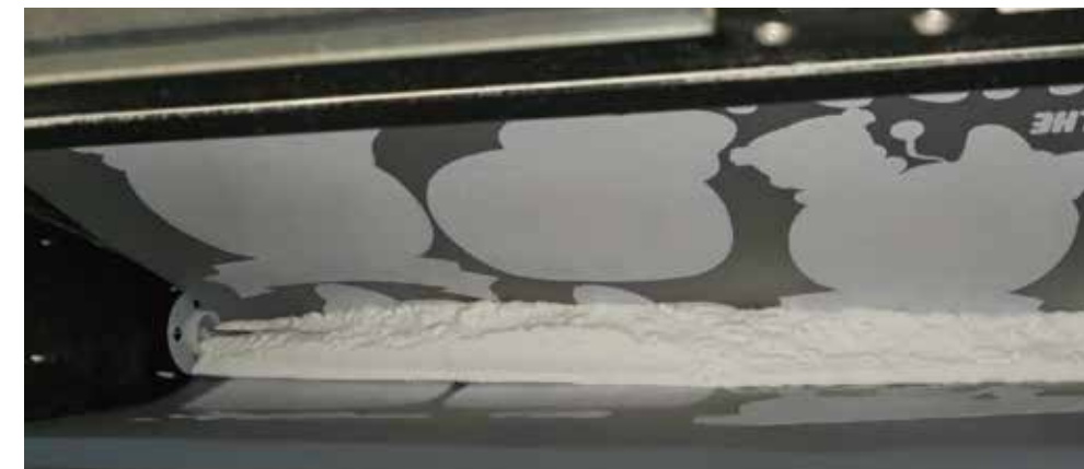
Powder stopping rod to make sure even powder supply
