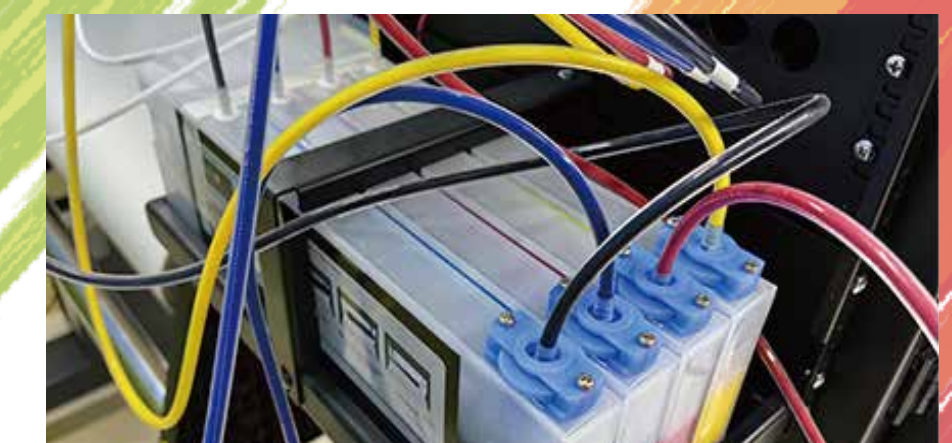
Independent ink cartridge stable ink supply
