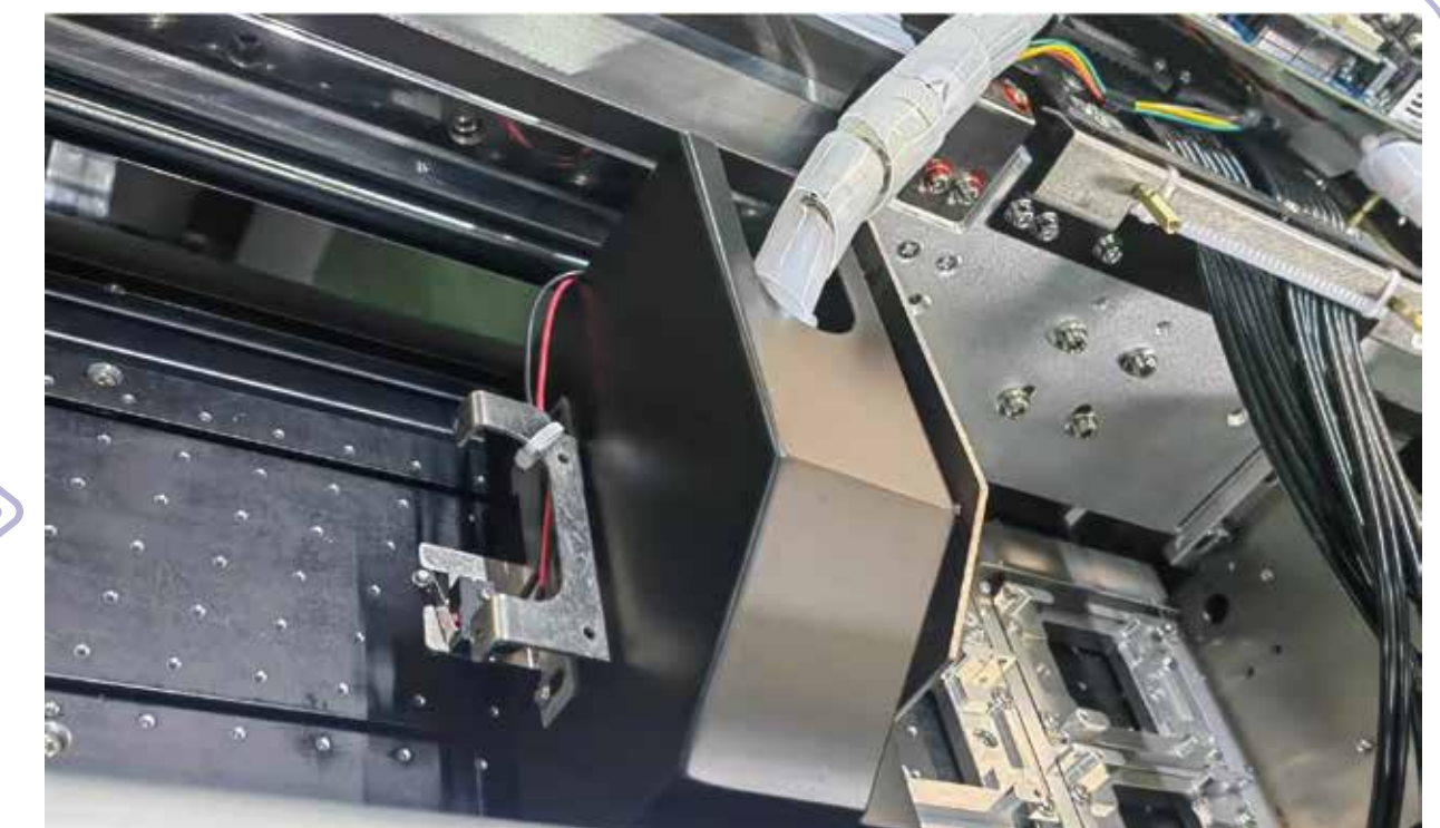
Head carriage anti-collision function
