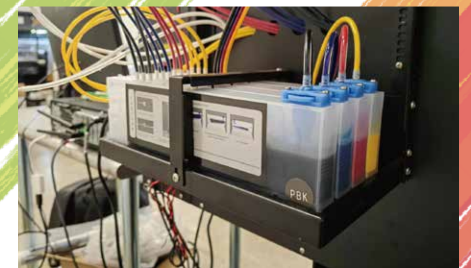
Stable ink delivery from secondary ink cartridges
