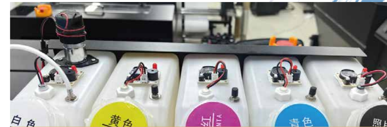
White ink stirring and circulation system Stirrer : avoid of head blocking Ink tank alarm device
