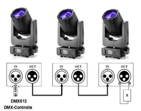
**DMX-512** Connection required terminal device (Loop connection)
