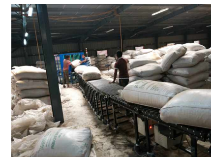
2.50kg茶叶袋仓库堆码输送线 50kg tea bags stacking and offloading conveyor system
