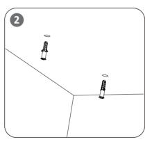
Drive the expansion screw into the drilled hole
