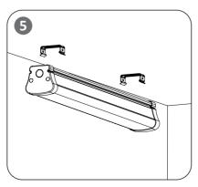
Hold the lamp and press it into the fastened buckle
