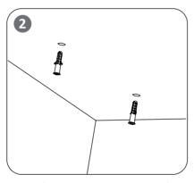
Drive the expansion screw into the drilled hole
