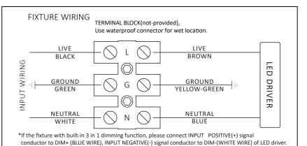
\*The junction box should have the same electrical hazard protection grade and IP rating with the luminaire
