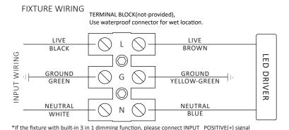
conductor to DIM+ (BLUE WIRE), INPUT NEGATIVE(-) signal conductor to DIM-(WHITE WIRE) of LED driver.
