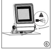
Note: The installation base must be able to support 10 times weight of the products
