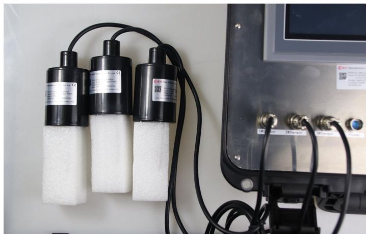
Soil moisture series sensor access
