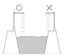
• The instrument shall be installed at least 20cm away from the side wall, and the underground pipe network shall be installed as close to the center of the well as possible, otherwise the well wall is prone to generate interference signals, affecting the measurement and judgment.
