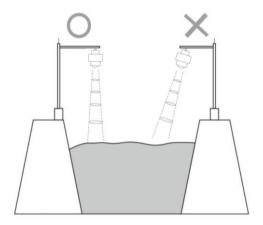
• Ensure that there are no interfering objects within the beam range, such as the riverbank.
