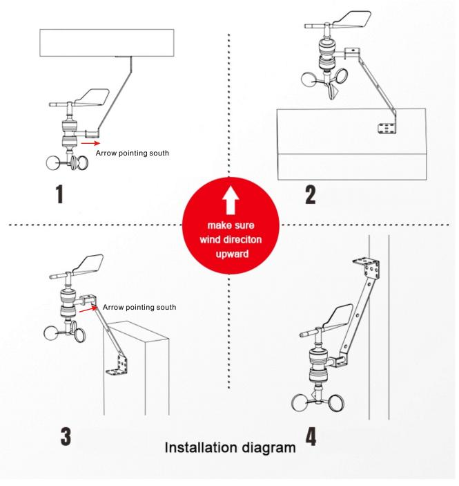
Ensure that the indicator arrow points south during installation
