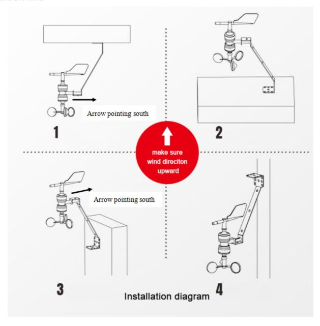
Ensure that the indicator arrow points south during installation
