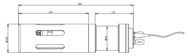
Note: Use lifting rings or pipe threads to install the sensor to avoid direct stress on the cable. The sensor connector is M16-5 cores male waterproof connector.
