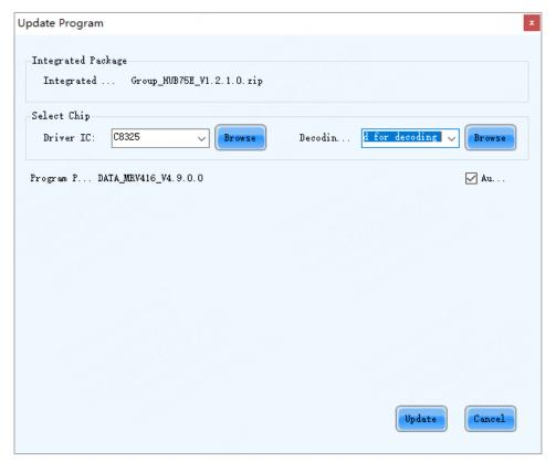
If the automatic match is not successful, users can manually select any program package and update the receiving card accordingly.
