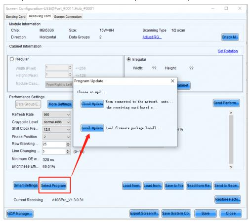
1. Cloud Update: Automatically matches the firmware package from the cloud based on the current configuration and updates the receiving card accordingly.
