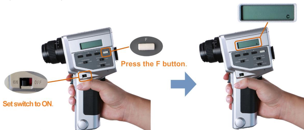
Figure 12-10 Setting CS-100A colorimeter
