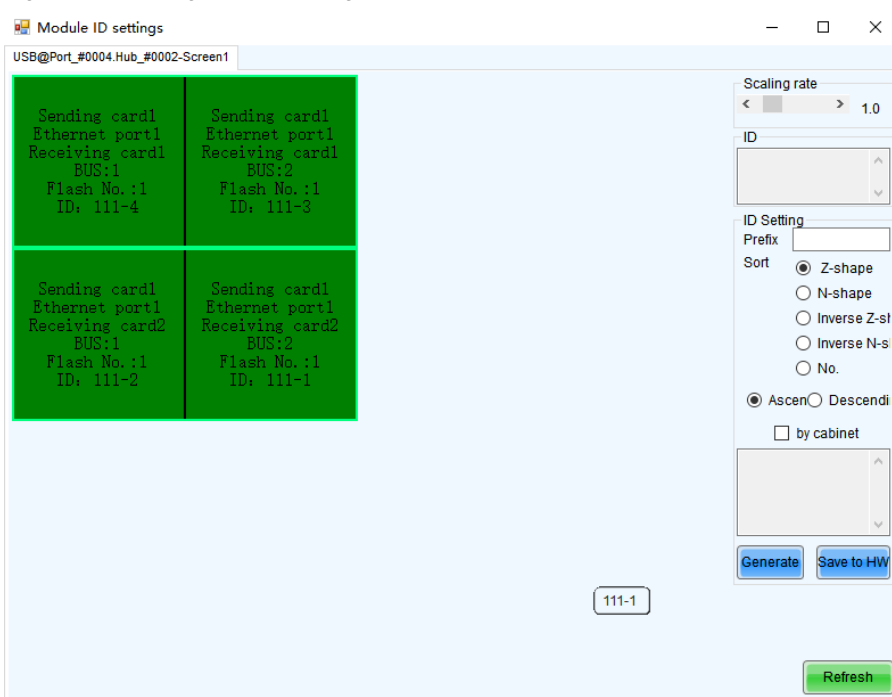
Figure 8-16 Setting module ID (regular screen)
