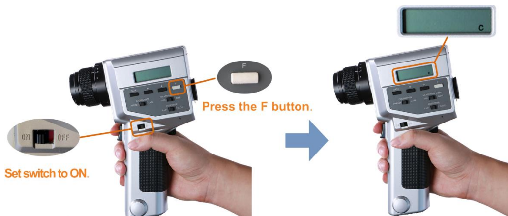
Figure 12-10 Setting CS-100A colorimeter
