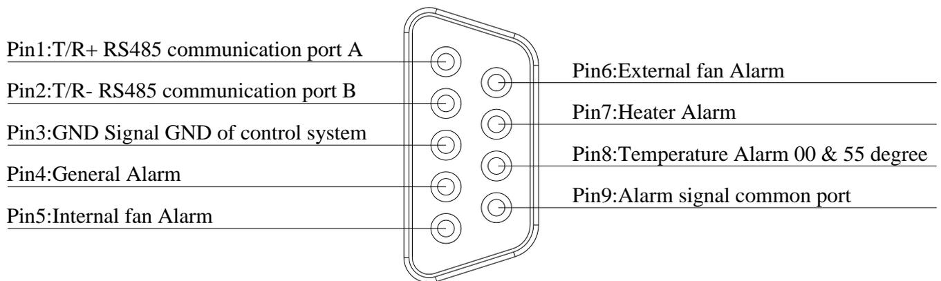
● Relay signal Output with no polarity dry switch type 无极性干节点继电器输出功能
