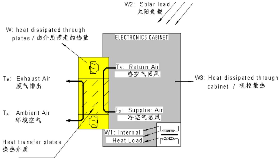
Heat exchanger is mostly used for enclosed area cooling, HRUC E series HEX is designed especially for mounting in a cabinet. The unit uses ambient air for temperature regulation so it must have access to ambient. The internal temperature of the enclosure is cooled via effective utilization of the ambient air. An air/air counter-current plate heat exchanger is used to transfer the heat. Two centrifuge fans, one for the internal circuit and one for the external circuit provide ventilation.
