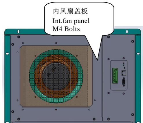
1. Unscrew the M4 bolts placed on the panel, then remove the panel; (see below pictures)
