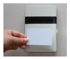
Reader is designed for close range reading, in order to read card one by one. With correct operating way and good position, the detecting success rate may reach 100%.
