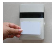
Reader is designed for close range reading/writing, in order to read/write card one by one. With correct operating way and good position, the writting success rate may reach 100%.
