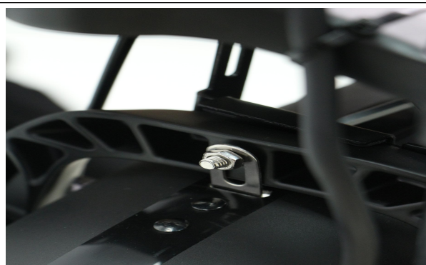
A24. details of the bolt that join headlight and fender together
