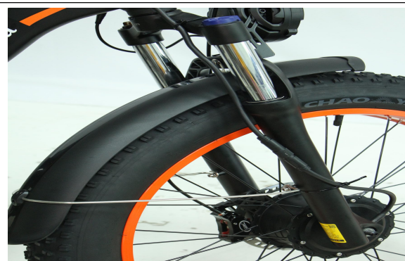
A25. The headlight and fender are fixed on the fork arch
