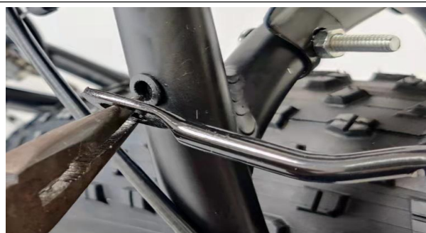
A32. Adjust the angles of the rack sticks with sharp-nose pliers
