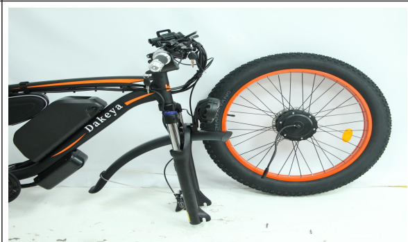
A12. Ready to install the front wheel
