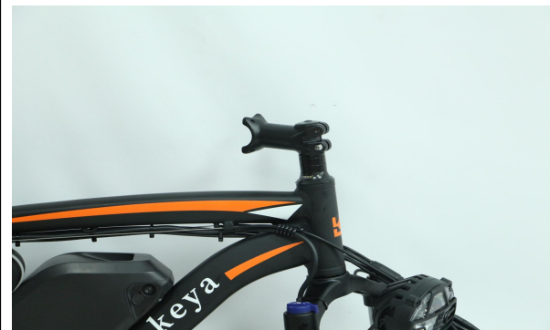
A03. The arch of the fork should be facing forward
