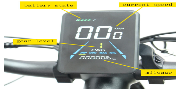
A42. LCD Display: battery status, real-time speed, speed grade, Mileage traveled
