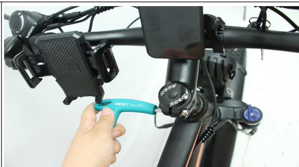
A10. Turn the 2 bolts on both sides to tighten the stem
