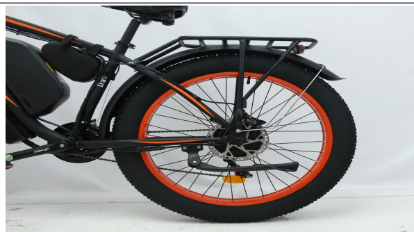
A26. Ready to install rear fender
