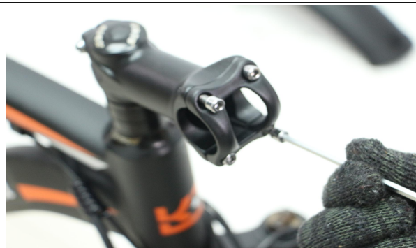
A05. The correct direction the stem should be facing
