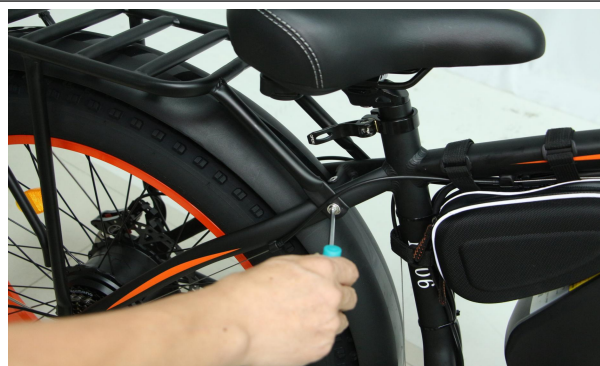
A33. Tighten the 2 upper bolts on both sides
