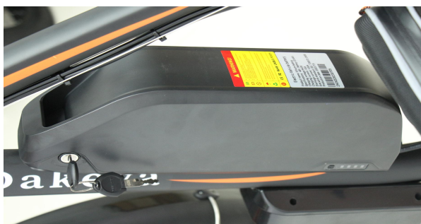
A39. Turn the key to lock the battery
