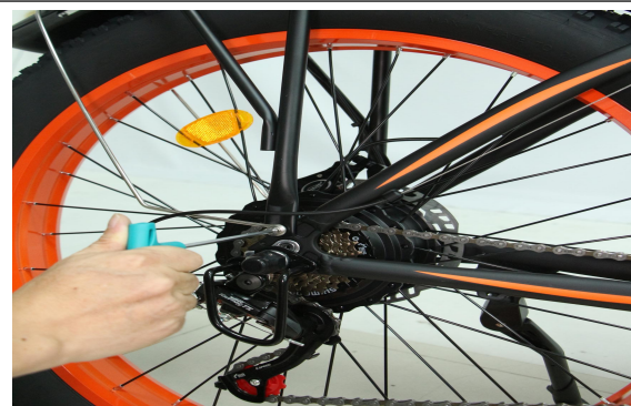
A34. Tighten the 2 lower bolts on both sides
