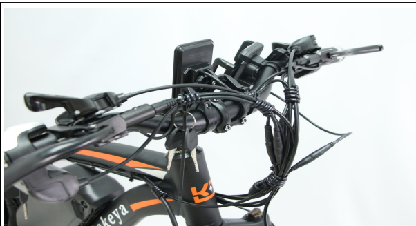
A09. Tighten the 4 bolts to fix handlebar
