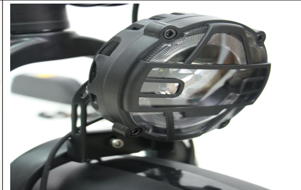
A23. Use the bolt to join the headlight, fork arch and fender
