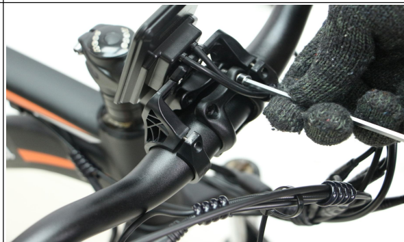
A08. Fit the stem and handlebar together
