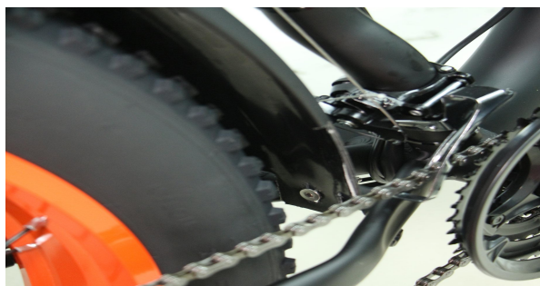
A28. Fix rear fender to the frame with bolt and nut
