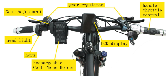
A41. Turn the key on the handlebar first and then press button Power ON/OFF for 3 seconds on the display to turn on power.
