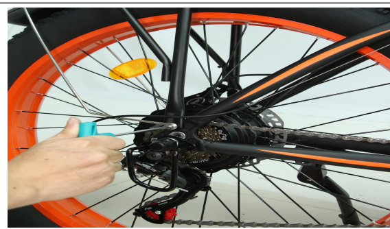
A27. The correct placement method of rear fender
