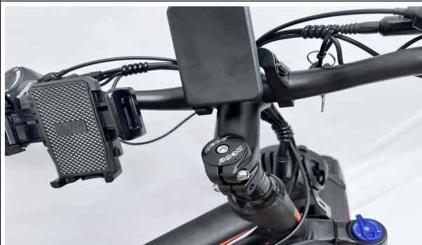
A11. Tighten the top bolt
