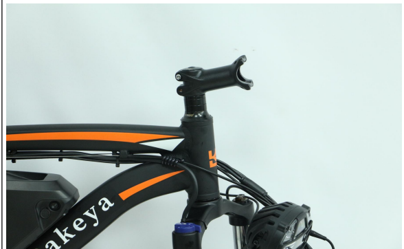
A04. Turn the stem forward ( do not turn the whole fork )
