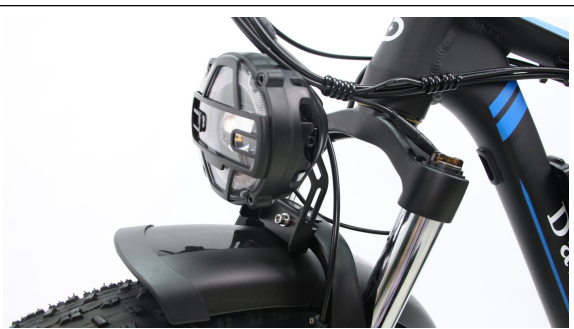
A23. Use the bolt to join the headlight, fork arch and fender
