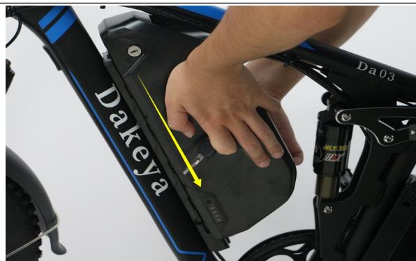
A37. Push the battery downward to install it tightly
