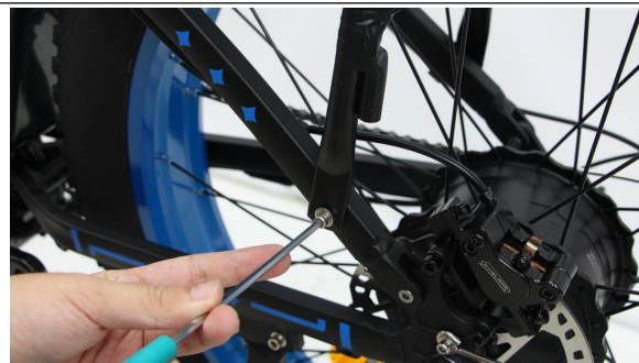
A33. Tighten the 2 lower bolts on both sides
