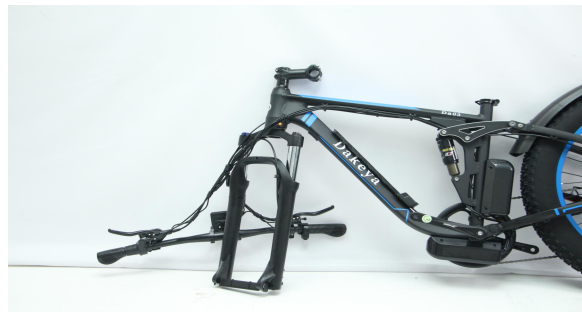
A03. The arch of the fork should be facing forward
