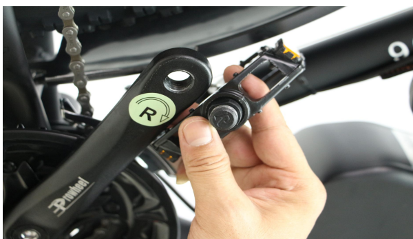
A35. Turn the spanner clockwise to fix the pedal R on the right side
