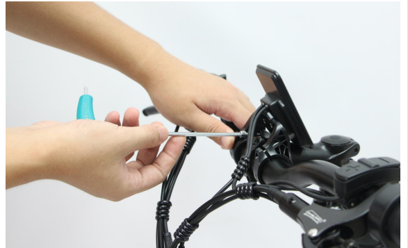
A08. Fit the stem and handlebar together
