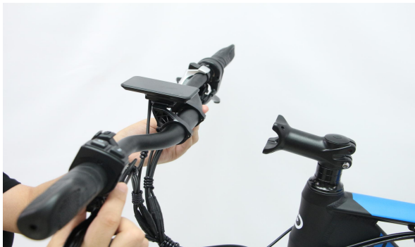
A07. The correct orientation of the handlebar
