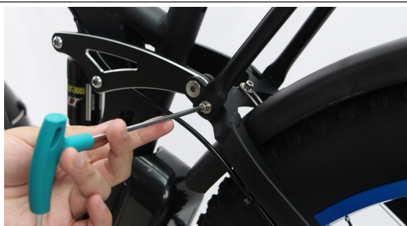
A32. Tighten the 2 upper bolts on both sides
