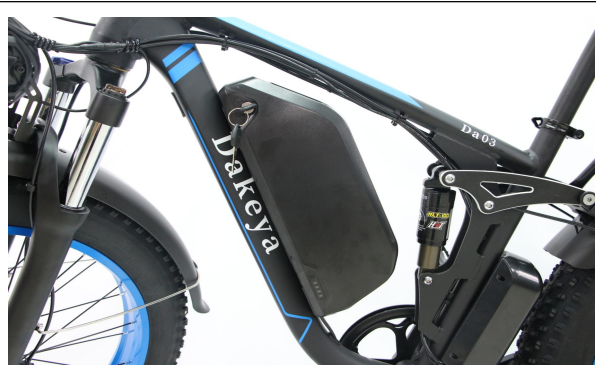
A38. Turn the key to lock the battery
