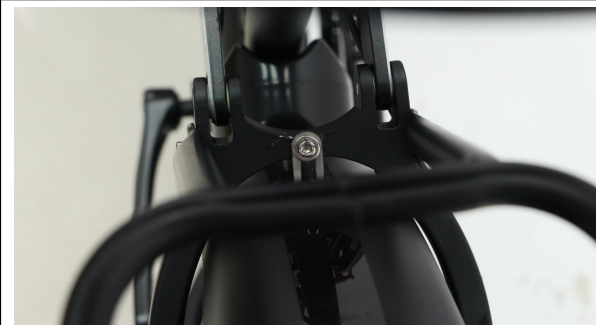
A28. Fix rear fender to the frame with bolt and nut
