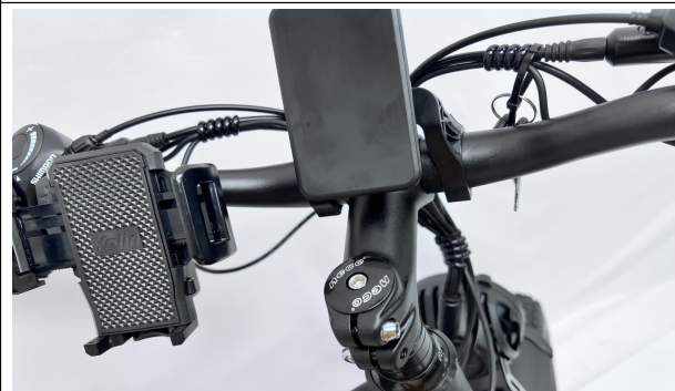
A11. Tighten the top bolt
