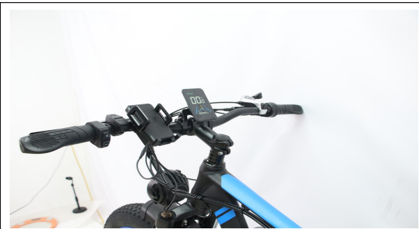
A09. Tighten the 4 bolts to fix handlebar
