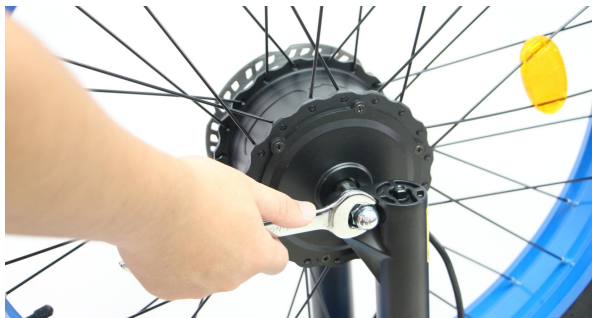
A18. Tighten the nuts on both sides
