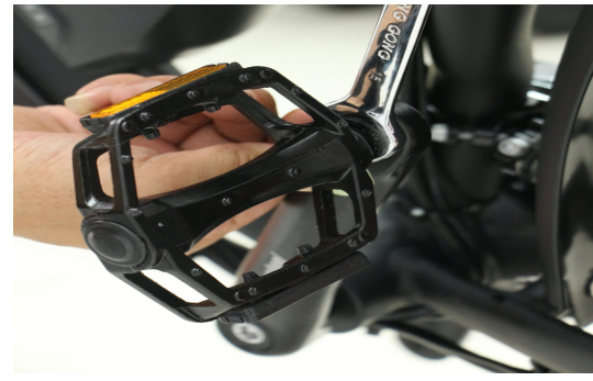
A34. Turn spanner counter-clockwise to fix the pedal L on the left side
