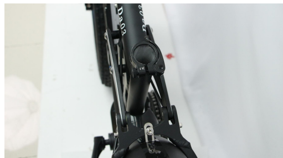
A19. Open the lever and turn the nut to loose the seat post clamp
