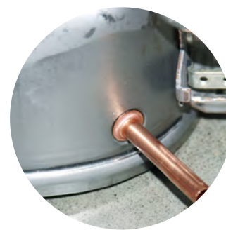
工艺管焊接 Welding Of Copper Tube
