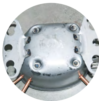
机脚焊接 Welding Of Base Legs
