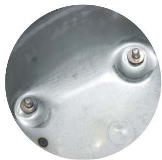
压簧支柱焊接 Welding Of Pins
