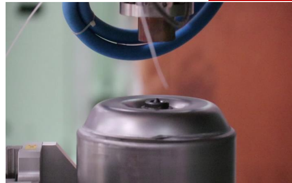
Resistance welding process for brake gas chamber
