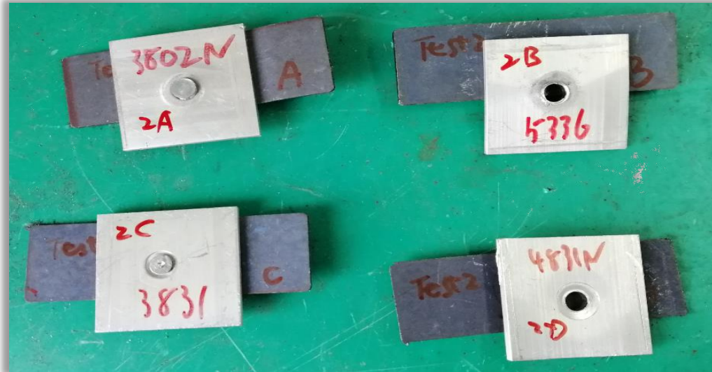
FSPR data reference of thermoformed steel + rolled aluminum plate
