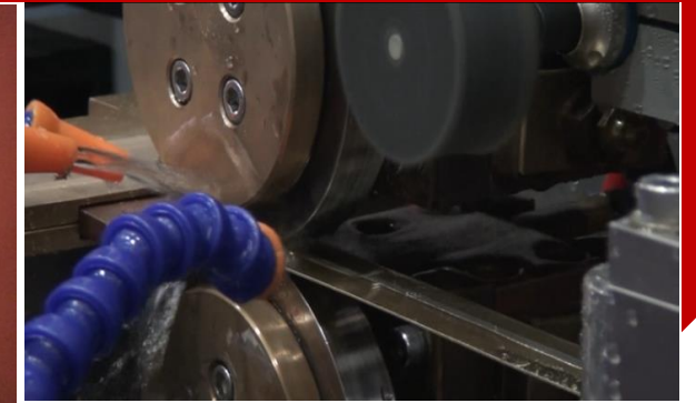
Resistance welding process for The connection of silver and copper
