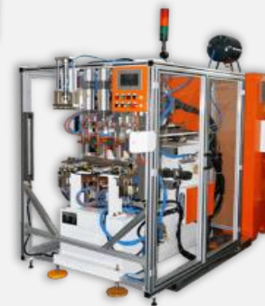
Door Frame BC Pillar Welding Equipment
