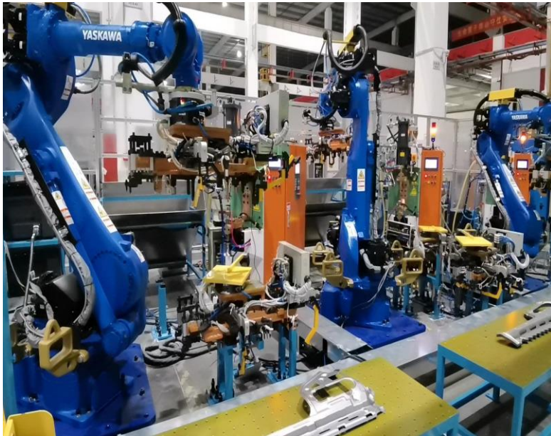
(Mid-sized Stamping Part) Projection Welding Station
