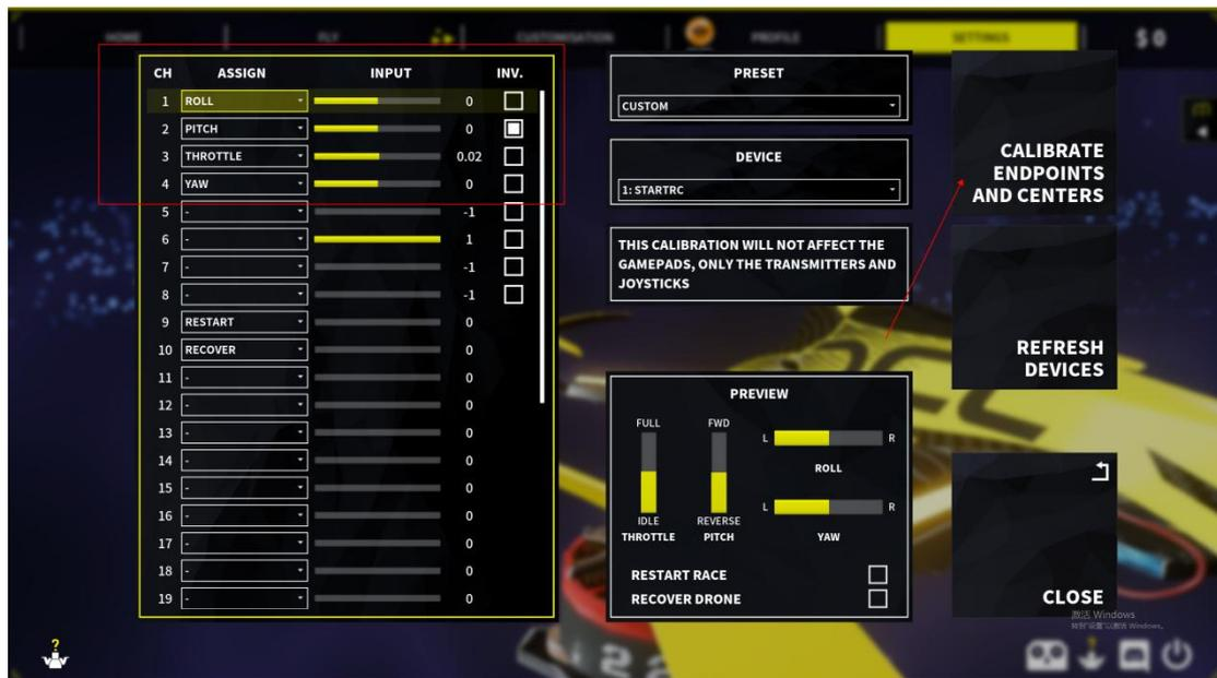
The corresponding channel allocation should be executed according to the diagram. If there is a problem with the joystick not returning to the center, you can follow the prompts in the "Calibration End and Return to Center" area on the right to complete the calibration.
