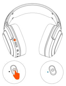
Long press the power button to turn on the headphones, press the mode switch button, and the blue light flashes to indicate that it is currently in Bluetooth mode.
