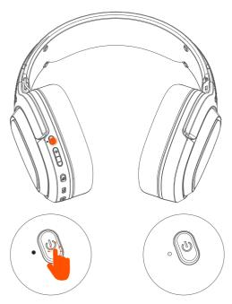
Long press the power button, the headphones will turn on, and a flashing white light indicates that the current mode is 2.4G.
