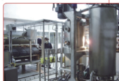
FCC: Flash vacuum chamber cooker 连续闪蒸蒸煮机
