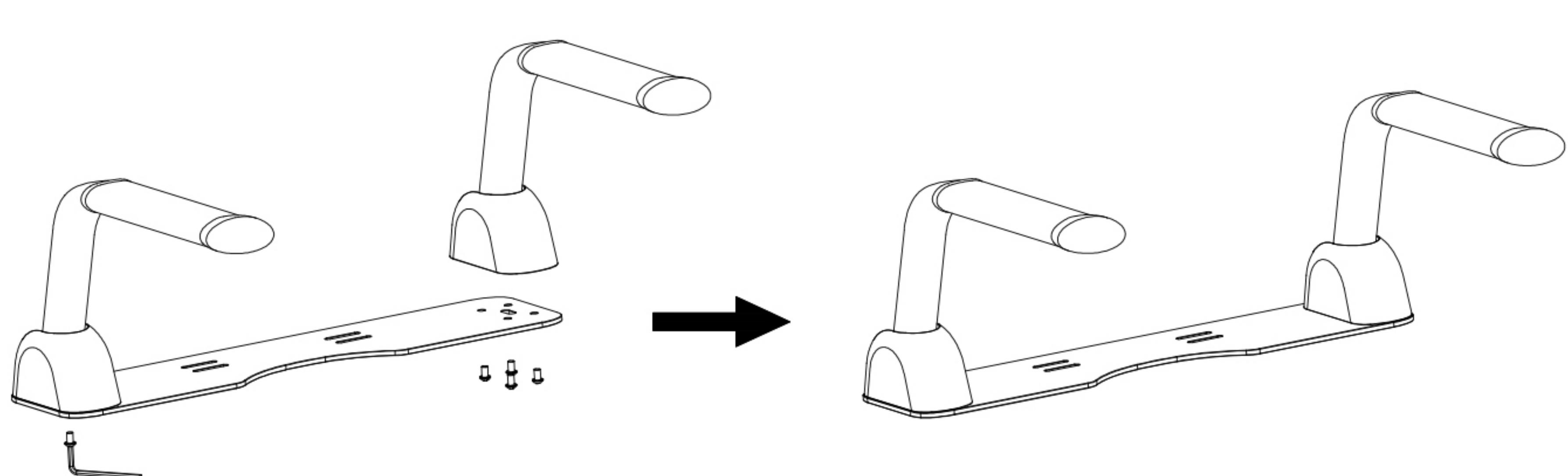
1. Install the handrail assembly, and lock the corresponding screws of the handrail assembly and the fixing plate with a M6 Allen screw, as shown in the figure above.
