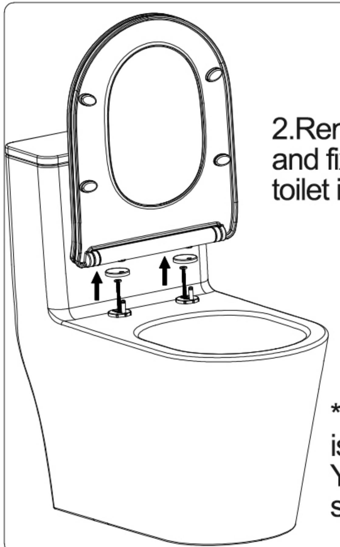
2. Remove the toilet seat and fixing device from the toilet in the correct way.
