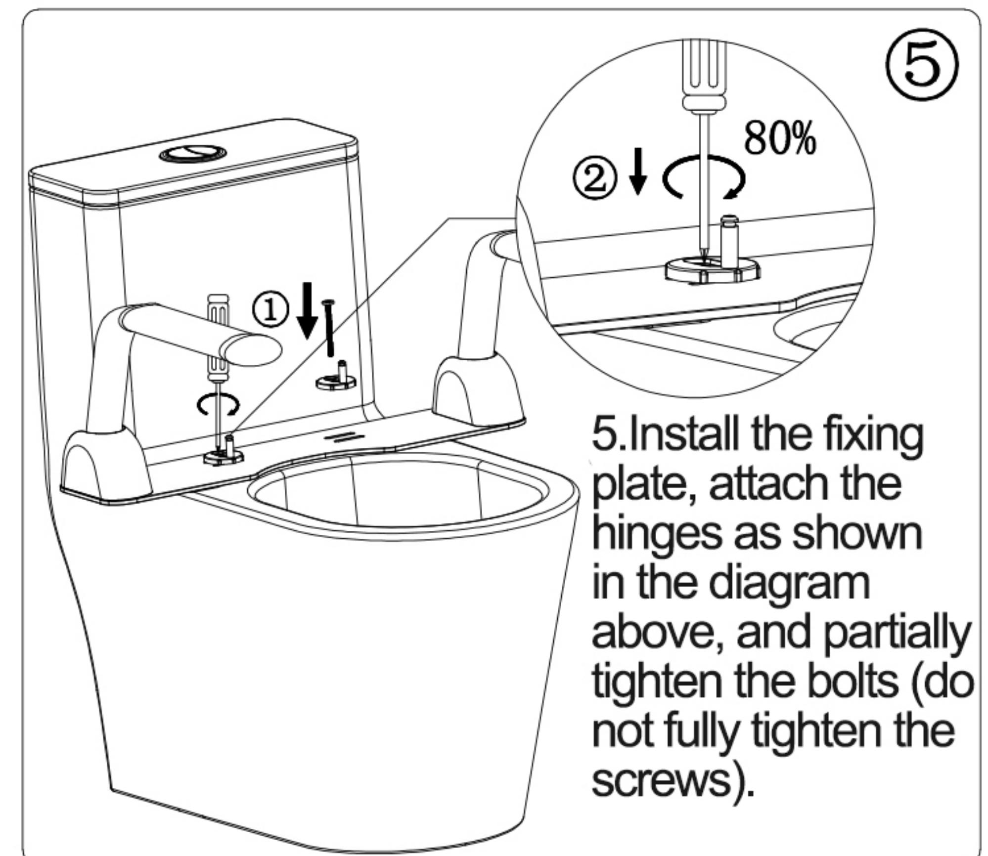
5. Install the fixing plate, attach the hinges as shown in the diagram above, and partially tighten the bolts (do not fully tighten the screws).
