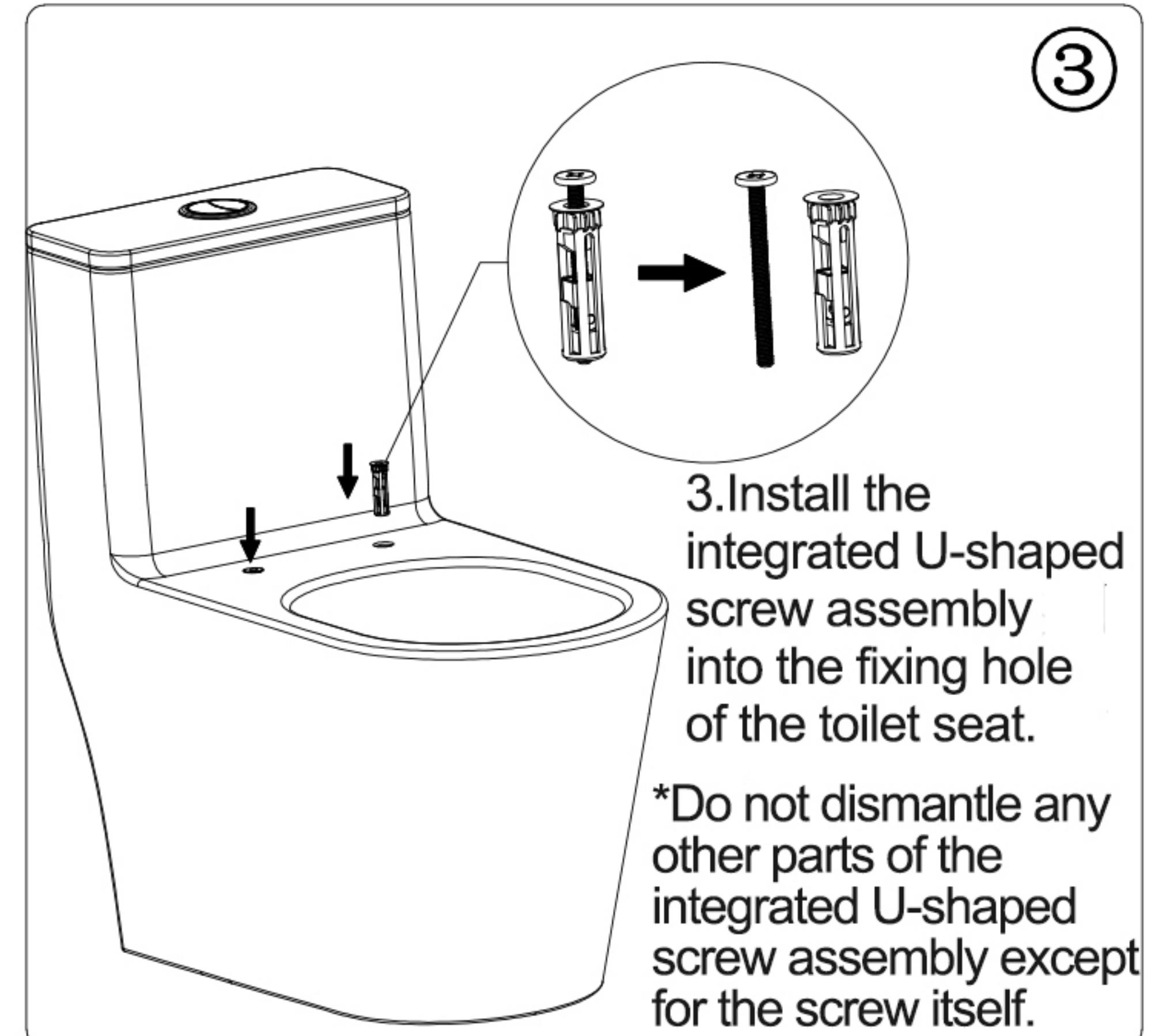
3. Install the integrated U-shaped screw assembly into the fixing hole of the toilet seat.
