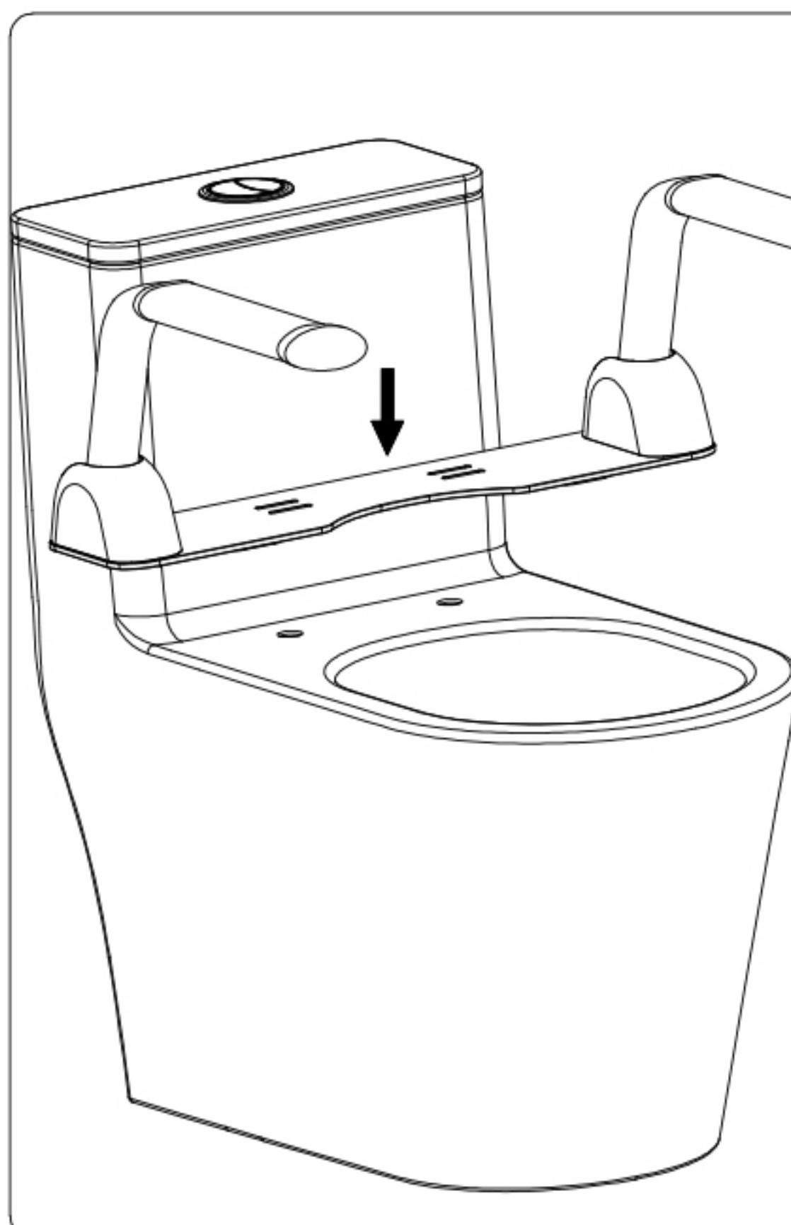
4. Place the fixing plate on the toilet and align the mounting holes of the fixing plate with the fixing holes on the toilet.
