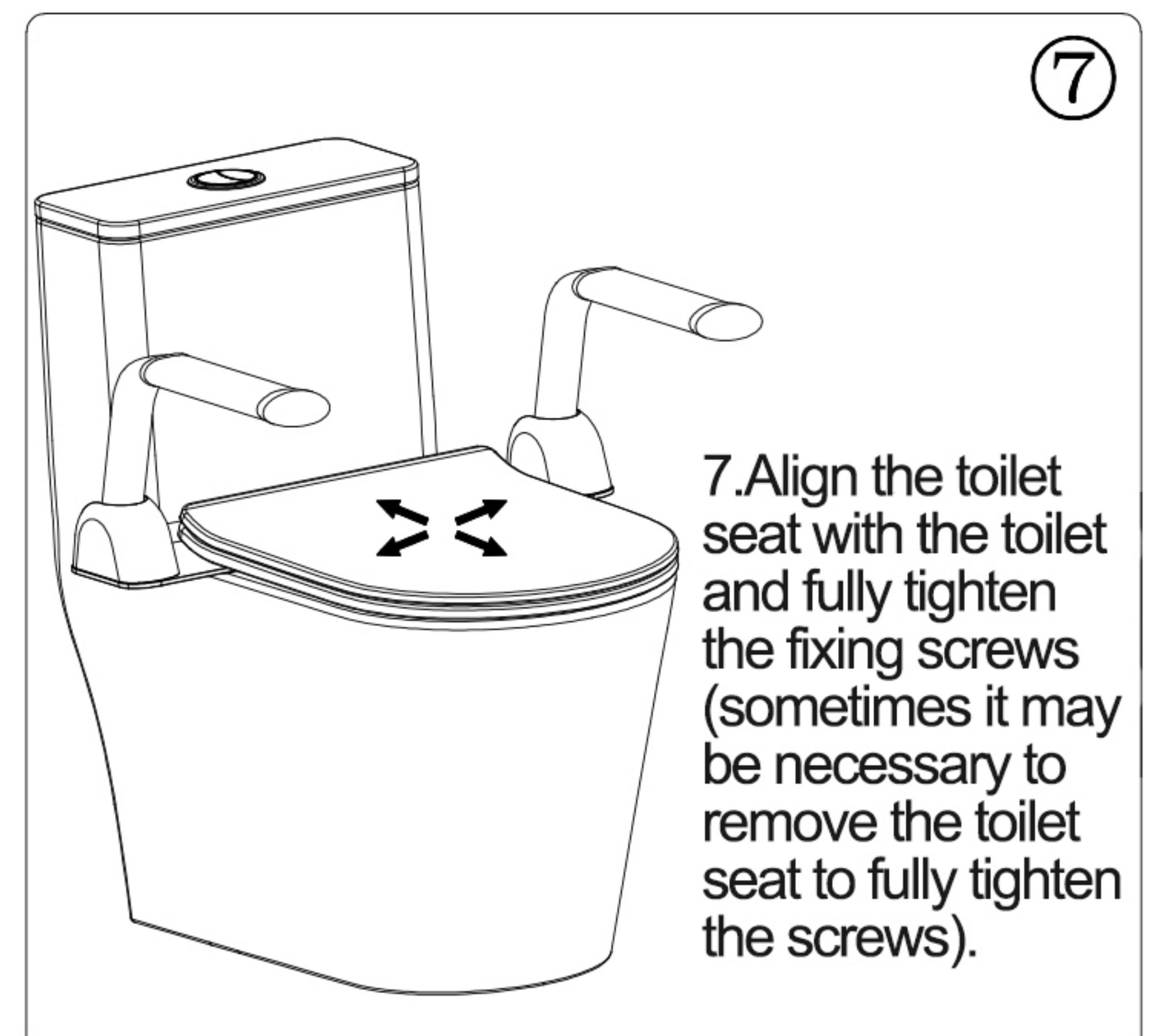
7. Align the toilet seat with the toilet and fully tighten the fixing screws (sometimes it may be necessary to remove the toilet seat to fully tighten the screws).
