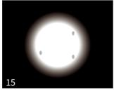
III. When small shadows or particles appear in the middle or edge of any spot (Figure 15, 16), open the lens and wipe the optical lens in Figure 8 with a dust-free cloth or eyeglass cloth
