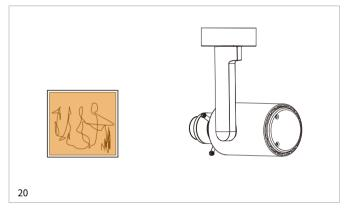
IV.Stretch the diaphragm sheet one by one outward until the spot size is substantially consistent with the object, as shown in Figure 20. If you are not satisfied with the effect, it is recommended to repeat the operation according to the above steps to bring up the spot effect you are happy with.
