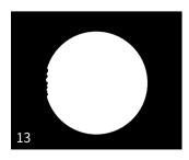
I .When the edge of the circular spot becomes rough or granular (Figure 13), please open the lens and wipe the red part in Figure 7 with a dust-free cloth or eyeglass cloth.
