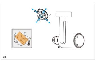
$\rm II$ . Pull the four diaphragm sheets outward to the maximum, and then push one by one vertically inward, to ensure that the cut square spot is smaller than the object to be illuminated, and adjust the sharpness of the aperture again until satisfactory, as shown in Figure 18.
