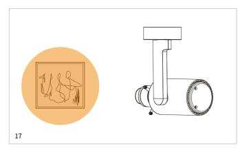
I .Adjust the aperture to the appropriate size, and facing the center of the irradiated object, adjust the sharpness to a reasonable degree, as shown in Figure 17.
