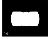
II .When the edge of the square spot becomes rough or granular (Figure 14), please open the lens and wipe the green edge in Figure 7 with a dust-free cloth or eyeglass cloth.
