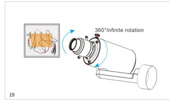
III. If the shape of the spot does not match the object to be illuminated, first loosen the hand screw at the red mark, rotate the blue part of the lens, adjust the edge of the spot to be parallel to the edge of the object to be illuminated, and finally tighten the hand screw. As shown in Figure 19, the LOGO projection direction not matching can also be adjusted to the ideal direction using this method.
