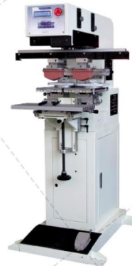
225-120PS2 2 color pad printer with pad shuttle
