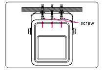
2 Install the bracket of the fixture in the screw of the solid part. As shown on the left.
