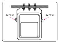
Connect the cables according to the wiring diagram on the left page and energize the lamps. Then adjust the screws on both sides of the lamp bracket according to the lighting angle.
